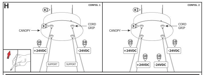
**NOTE:** Cord grips hold the fixture weight only. **DO NOT** pull on the fixture during installation or cleaning which may cause the **power wires to nick and short**.
