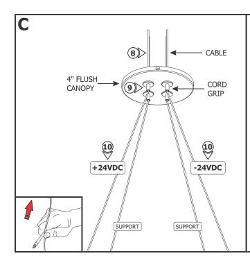
**NOTE:** Cord grips hold the fixture weight only. **DO NOT** pull on the fixture during installation or cleaning which may cause the **power wires to nick and short**.
