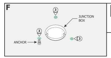
**NOTE:** Step 3 is for drywall mounting. Omit this step if mounting directly to wood surface.
