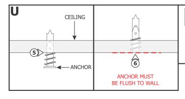
**NOTE:** Steps 5 and 6 are for drywall mounting. Omit these steps if mounting to a wood surface directly.
