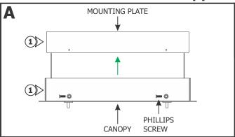
1: Remove the four Phillips screws from the canopy to remove the mounting plate.
