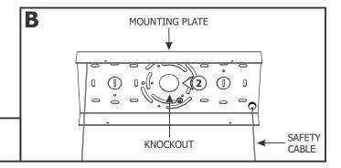
2: Select the appropriate knockout on the mounting plate and remove it using a flathead screwdriver or other appropriate
