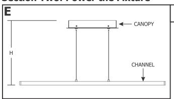
**1:** Determine the fixture height (H), from the bottom of the channel to the top of the canopy.
