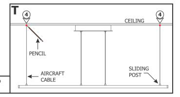
**4:** Lift the other end of the aircraft cables against the ceiling to mark the location of the standoffs.
