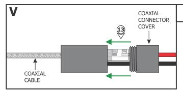
**13:** Replace the coaxial connector cover and tighten into place.
