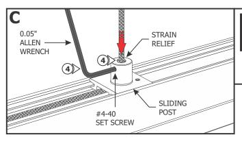
**<u>!CAUTION!</u>** Tightening the strain relief set screw **CANNOT BE REVERSED**. Only tighten the set screw AFTER the cable location is set properly.
