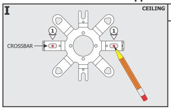
1: Mark the points through the crossbar holes onto the ceiling. These points are used for the anchors.
