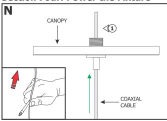
1: Feed the coaxial cable through the canopy.
