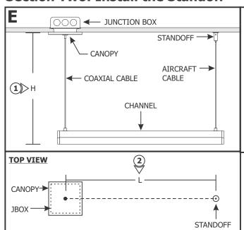
**NOTE:** Run the proper size wires between the 24VDC power supply to the electrical box. Refer to the instructions provided with the power supply for additional information.
