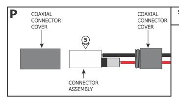
**5:** Unscrew the coaxial connector covers and remove from the connector assembly.
