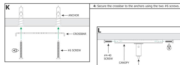
5: Align the canopy with the crossbar and secure it using the two #4-40 screws using a 1/16" Allen wrench.
