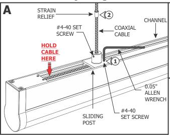
**WARNING:** To avoid damaging the coaxial cable electrical connection, make sure that the end of the coaxial cable coming out of the fixture is held with thumb before relocating sliding posts.
