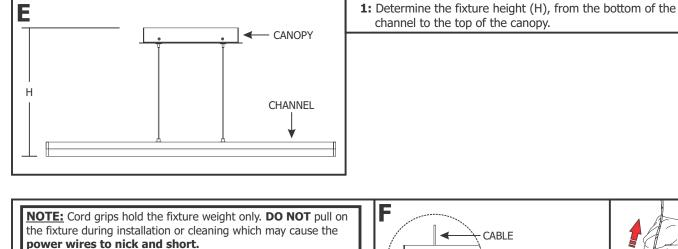
**NOTE:** If cable is curled or kinked, straighten by holding between the shaft of a screwdriver and thumb and pulling the cable through.
