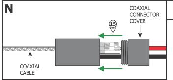
**15:** Replace the coaxial connector cover and tighten into place.
