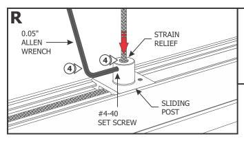
**!CAUTION!** Tightening the strain relief set screw **CANNOT BE REVERSED**. Only tighten the set screw AFTER the cable location is set properly.
