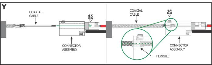
**10:** Insert the coaxial cable into the coaxial connector until the wires of the center conductor are visible through the M3 set screw hole.
