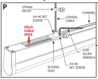
**WARNING:** To avoid damaging the coaxial cable electrical connection, make sure that the end of the coaxial cable coming out of the fixture is held with thumb before relocating sliding posts.
