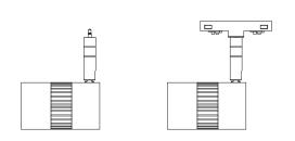
1: Unscrew the lens holder counter-clockwise and remove it
