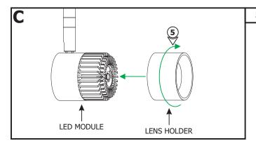
**5:** Screw the lens holder back clockwise to secure in place.
