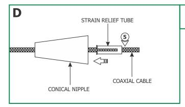
**5:** Feed the coaxial cable through the conical nipple and flared side of the strain relief tube. Slide the conical nipple and strain relief tube down the coaxial cable.
