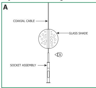
**2:** Cut the coaxial cable to the desired height (H) with a sharp cutter. The overall fixture height is measured from the bottom of the glass shade to the end of the coaxial cable.
