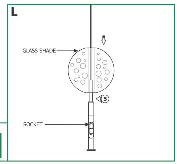
**5:** Carefully lower the glass shade onto the socket assembly.
