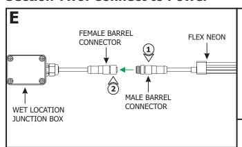
**NOTE:** Outdoor electrical connections must be made inside a waterproof junction box or using waterproof wire nut connections.
