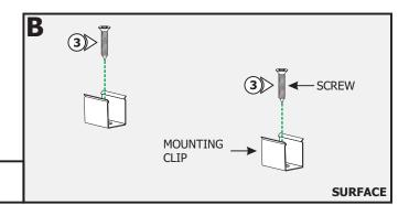
**3:** Secure the mounting clips to a wood surface by tightening the screws to each clip.
