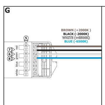
**NOTE:** The color of the power cord wires are represented as:
