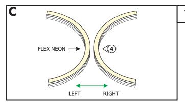
**4:** If necessary, bend the Flex Neon **ONLY** right to left or left to right.
