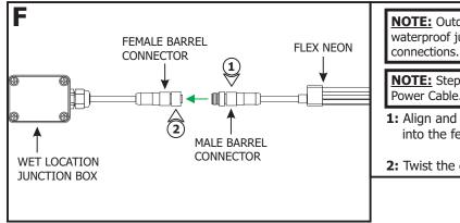
**NOTE:** Outdoor electrical connections must be made inside a waterproof junction box or using waterproof wire nut connections.
