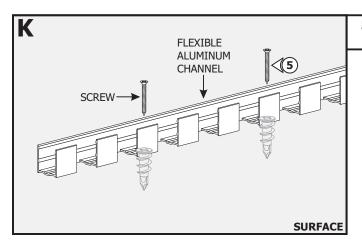
**5:** Secure the Flexible Aluminum Channel to the anchors using screws.
