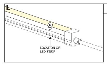
**6:** Identify the side of the Flex Neon with a white stripe that indicates the location of the LED Strip.
