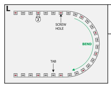
**2:** Determine the location of the Flexible Aluminum Channel and mark every fourth tab screw holes.
