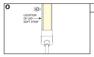
**6:** Identify the thicker side of the Flex Neon that indicates the location of the LED Soft Strip.
