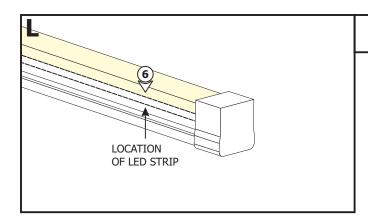
**6:** Identify the side of the Flex Neon with a thin white strip that indicates the location of the LED Strip.
