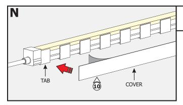
**10:** Remove the backing from the channel cover. Firmly press down on the Flexible Aluminum Channel tabs while removing the rest of the backing.
