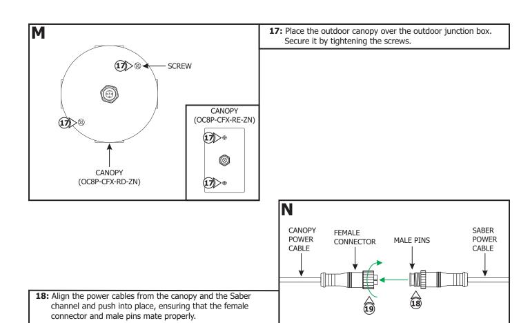
19: Twist the connector nut to lock in place.
