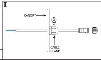
**3:** Insert the power cable through the outdoor canopy and tighten the waterproof cable gland to lock in place.
