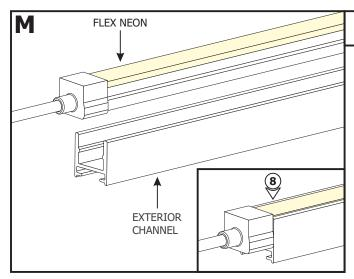
8: Push the Flex Neon inside the Exterior Channel, leaving the end cap outside of the Exterior Channel.
