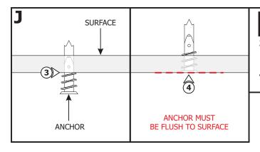
**NOTE:** Steps 3 and 4 are for drywall mounting. Omit these steps if mounting to a wood surface directly.
