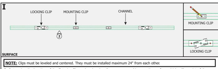
**2:** Determine the location of the Exterior Channel and make all necessary markings on the surface which will consist of the sides and center of the Exterior Channel, mounting clips and locking clips.
