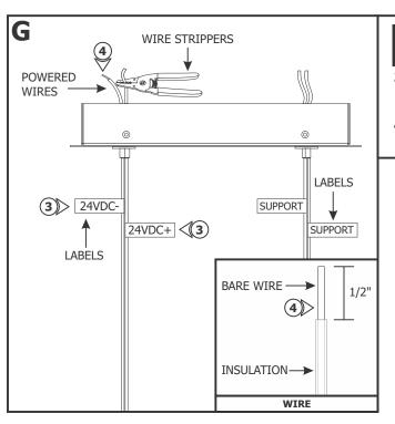
**NOTE:** The wires with "SUPPORT" labels are the support wires. **DO NOT** strip and power the support wires.
