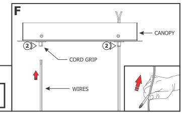
**2:** Split the end of the wires and push the wires through each tab on the cord grip of the canopy.
