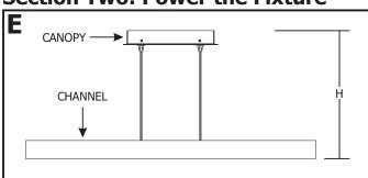
**1:** Determine the fixture height (H), from the bottom of the channel to the top of the canopy.
