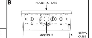
2: Select the appropriate knockout on the mounting plate and remove it using a flathead screwdriver or other appropriate tool.
