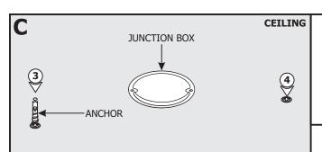
3: Align the mounting plate holes with the junction box. Mark one point on each side of the junction box onto the ceiling.
