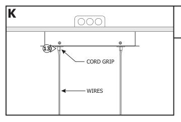
13: To make any adjustments to the fixture height, push the cord grips to slide the fixture up and down until the desired height is achieved. Release the cord grips to lock the wires in place.
