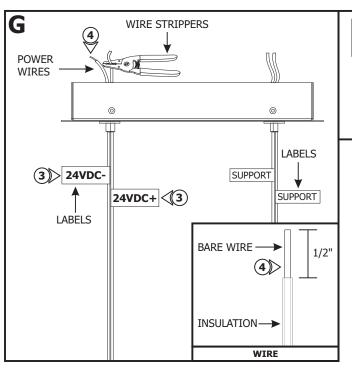
**NOTE:** The wires with **"SUPPORT"** labels are for support only. **DO NOT** strip and power the support wires.
