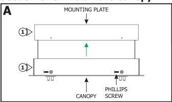
1: Remove the four Phillips screws from the canopy to remove the mounting plate.
