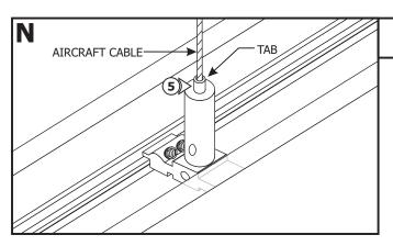
**5:** Insert the aircraft cable through the top of the tab on the sliding post.
