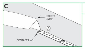
**3:** Place the LED strip on a flat, stable surface. Using a utility knife, carefully scrape the protective coating from the contacts on both ends.
