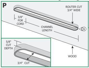
**1:** Determine the location for the Light Channel .6 Millwork on the wood.
