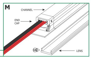
**16:** Snap the lens(es) to the assembled channel(s).
