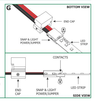
**8:** Insert the LED strip into one end of the Snap & Light Power/Jumper connector so that the "24VDC+" mark on the strip is aligned with the red wires. Ensure the LED strip contacts align fully with the contact pins. Push the LED strip completely into the contact pins.
