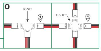
**4:** Refer to steps 1 through 3 if using the Light Channel Snap & Light X-Connector or T-Connector (sold separately).
