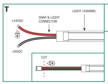
**6:** Cut the other end of the power cord that is going to be connected to power and discard the unused connector. Strip the ends of the wires.
