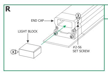
**3:** Insert the light block into the end cap. Secure the light block by tightening the two #2-56 set screws using a 0.035" Allen wrench.
