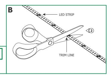
**NOTE:** Do not trim the strip at unmarked sections which may cause that section of the strip not to light up.
