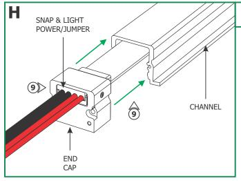
**9:** Insert the Snap & Light Power/Jumper connector inside the end cap and place the end cap onto the channel.
