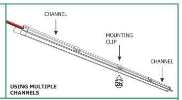
2a: Snap the light channel assembly to the mounting clips. Mounting clips must be maximum 24" apart from each other.
