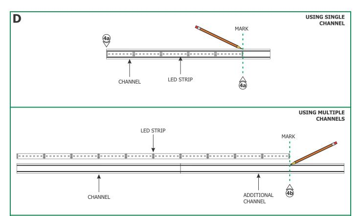
**4a:** If using a single channel, lay the LED strip inside the single channel flush to one end and mark the length of the LED strip on the channel.
