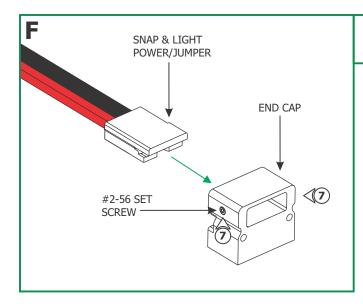
7: Loosen (**Do Not Remove**) the two #2-56 set screws on the end cap using a 0.035" Allen wrench. Insert the Snap & Light Power/Jumper Connector through the end cap.
