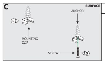
**5:** Align the mounting clips to the anchors and secure each clip to each anchor by tightening the #8 screws.
