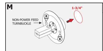
8: Place the turnbuckle into the hole and mark the two screw holes.
