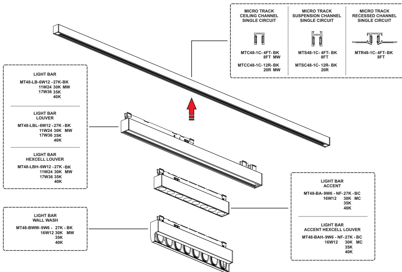
**1:** Determine the location of the Light Bar on the track. Push the Light Bar into the track.
