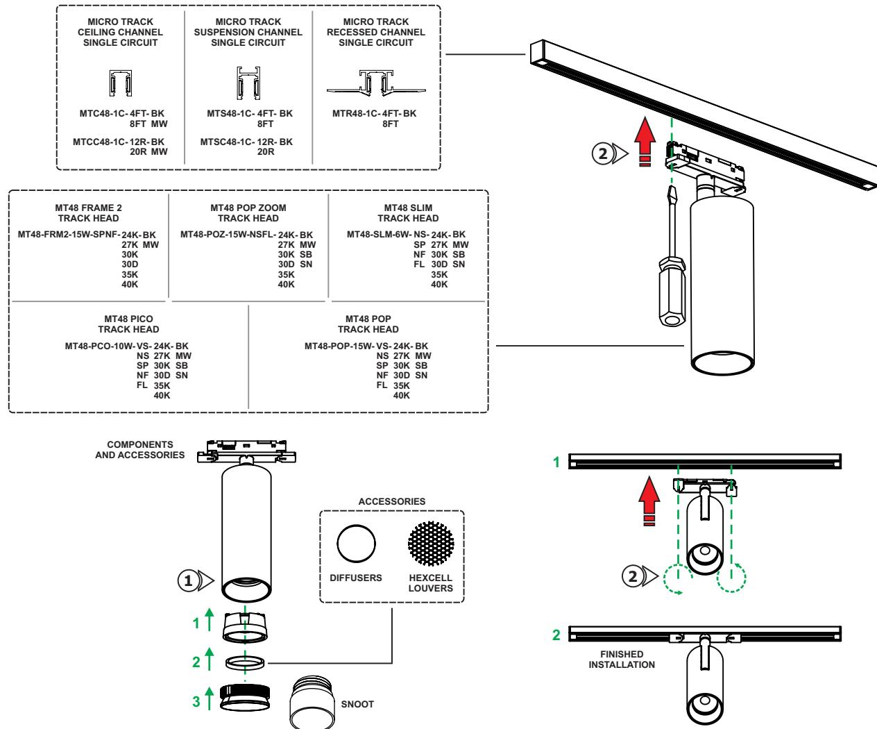
**1:** If necessary, unscrew the lens holder or snoot. Replace the lens or replace the accessory. Place the accessory in front of the lens and screw the lens holder or snoot back into the fixture to secure in place.
