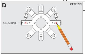
**1:** Mark the points through the crossbar holes onto the ceiling. These points are used for the anchors.
