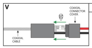
**17:** Replace the coaxial connector cover and tighten into place.
