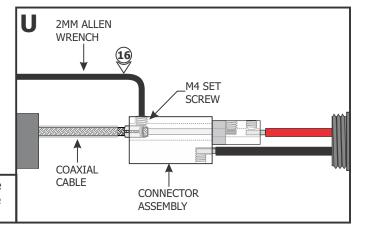
**16:** Use the provided 2mm Allen wrench to securely tighten the M4 set screw until it squeezes the wire ferrule tightly to the coaxial cable.
