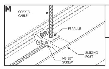
**<u>iCAUTION!</u>** Tightening the ferrule set screw **CANNOT BE REVERSED.** Only tighten the set screw AFTER the cable location is set properly.
