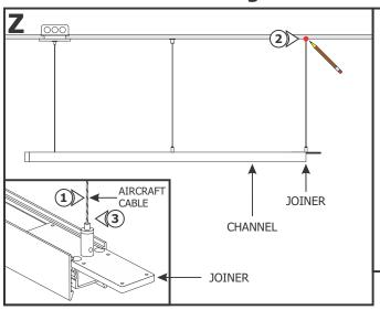
**NOTE:** If applicable, multiple channels must be installed one by one.
