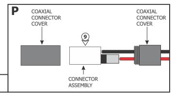
**9:** Unscrew the coaxial connector covers and remove from the connector assembly.
