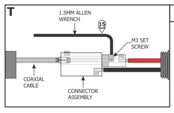
**15:** Use the provided 1.5mm Allen wrench to replace and securely tighten the M3 set screw.
