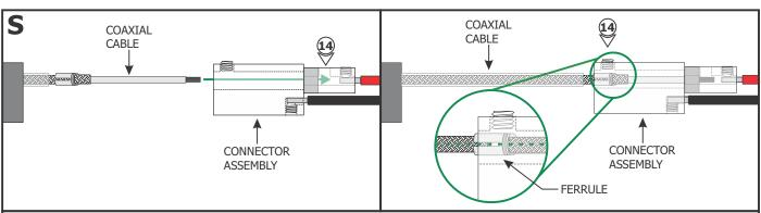
**14:** Insert the coaxial cable into the coaxial connector until the wires of the center conductor are visible through the M3 set screw hole.
