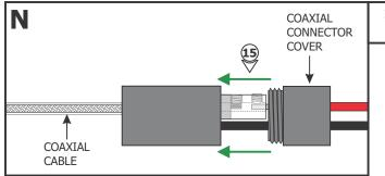
**15:** Replace the coaxial connector cover and tighten into place.
