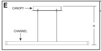
**1:** Determine the fixture height (H), from the bottom of the channel to the top of the canopy.
