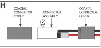
**7:** Unscrew the coaxial connector covers and remove from the connector assembly.
