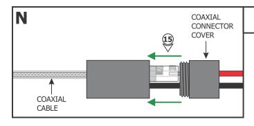
15: Replace the coaxial connector cover and tighten into place.
