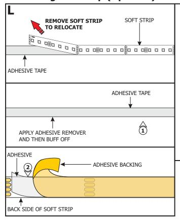
**NOTE:** If relocating the installed soft strip, make sure that the adhesive tape on back of the soft strip covers the entire strip. The adhesive tape isolates the strip from the installation surface. Damaged or inconsistent adhesive tape may cause the contacts on the back of the strip to come in contact with the conductive heat sink which will cause the strip to short and burn. Call PureEdge Lighting to get replacement adhesive tape and/or optional aluminum heat sink tape (SS-HR-F).
