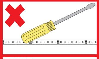
**DO NOT** use any tool to install soft strip to a surface. This will damage the soft strip component.
