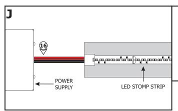
**16:** Trim the other end of the Snap & Light connector when it is used as the power cord.
