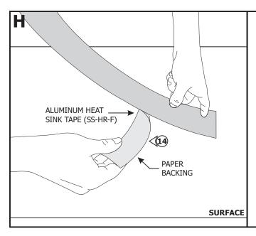
**NOTE**: It is recommended to use the provided heat sink tape with ST7A and ST10A.
