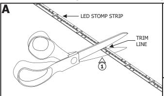
1: If necessary trim the LED strip at the marked line above the contact (every 2.4" apart) with a sharp scissor to fit the desian.
