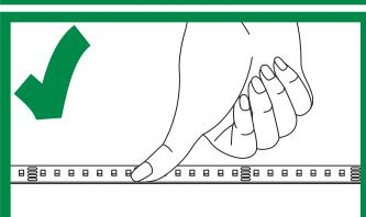
**DO** only ever use fingers to gently install soft strip to a surface **AFTER** cleaning the surface with alcohol.
