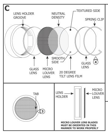
3: Carefully remove the spring clip and one of the glass lenses.
