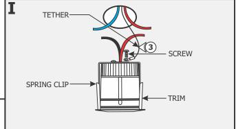
**3:** After installing drywall and finishing it, align the tether terminal to the trim tab and secure it by replacing the Phillips screw.
