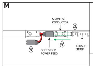
**NOTE:** LED Strip may not properly adhere to channel surface unless the channel is cleaned with alcohol prior to application.
