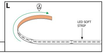
**2:** Gently uncoil the LED Soft Strips before applying to the channel otherwise the strip may lift off of the surface.
