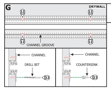
12: Place the assembled channel in the drywall cutout. Using the marked joist and mounting strap locations on the drywall, drill and countersink the channel along the groove lines using the provided square drill with countersink bit.
