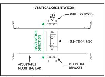
1: Mount each adjustable mounting bar to one side of the junction box and secure them with the mounting brackets and Phillips screws provided.
