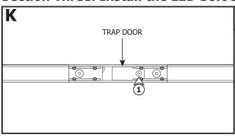
**1:** Secure the trap door to the Center Power Feed with the provided set screw using an Allen wrench.
