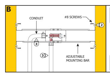
**NOTE:** Adjustable mounting bars mount to studs that are spaced 15" to 24" apart. If the span needs to be shorter than 15", then break the bar arms from dedicated lines.
