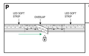
**8:** If using one Soft Strip Power Feed and routing LED Soft Strip from other power feeds, trim excess LED Soft Strip from the other power feeds **ONLY** at dashed cutting lines and overlap it with the other LED Soft Strip at power connection to avoid dark spots in the installation.
