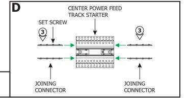
**3:** Insert the joining connectors half way into the Center Power Feed Track Starter and tighten the set screws using the provided Allen wrench.
