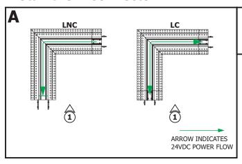
1: L-Connectors join two track sections together in a 90 degree angle and either isolate the power from one track to the other (LNC) or conduct the power from one track to the other (LC).
