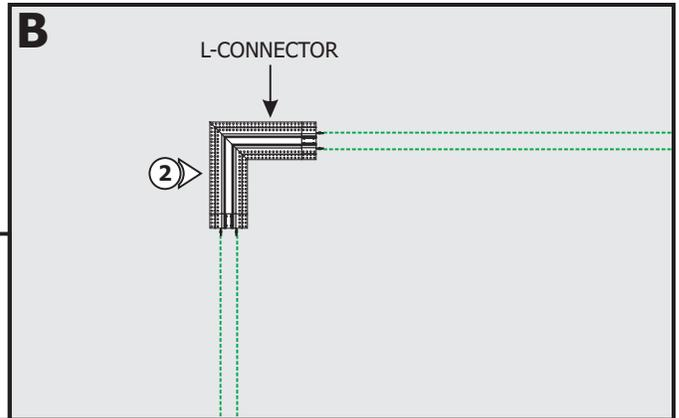
**2:** Place the L-Connector against the ceiling. Ensure the L-Connector is aligned with the TruTrack Recessed Channel installation location.
