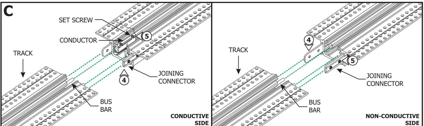
**4:** Slide the track over the joining connectors on the conductive or non-conductive side of the connectors.
