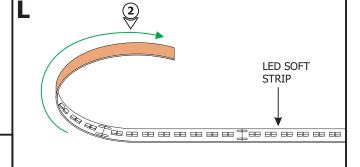
**2:** Gently uncoil the LED Soft Strip before applying to the channel otherwise the strip may lift off of the surface.
