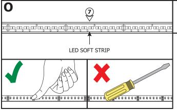
7: Firmly press down the adhesive portion of the LED Soft Strip onto the track surface while removing the rest of the backing, making sure there are no air bubbles that can cause surface irregularities.
