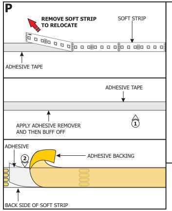
**NOTE:** If relocating the installed soft strip, make sure that the adhesive tape on back of the soft strip covers the entire strip. The adhesive tape isolates the strip from the installation surface. Damaged or inconsistent adhesive tape may cause the contacts on the back of the strip to come in contact with the conductive heat sink which will cause the strip to short and burn. Call Edge Lighting to get replacement adhesive tape and/or optional aluminum heat sink tape (SS-HR-F).
