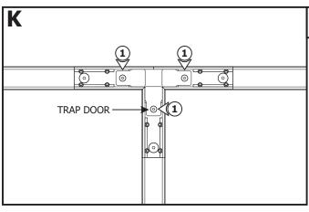
**1:** Secure the trap doors to the T-Shaped Power Feed with the provided set screws using an Allen wrench.
