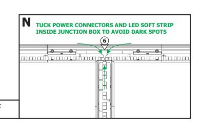
**6:** Place the Soft Strip Power Connectors or excess LED soft strips inside the junction box to avoid dark spots.
