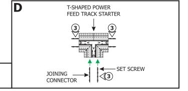
**3:** Insert the joining connectors half way into the T-Shaped Power Feed Track Starter and tighten the set screws using the provided Allen wrench.
