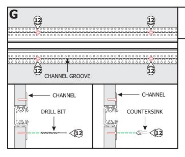
**12:** Place the assembled channel in the drywall cutout. Using the marked joist and mounting strap locations on the drywall, drill and countersink the channel along the groove lines using the provided square drill with countersink bit.
