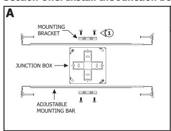
**1:** Mount each adjustable mounting bar to one side of the junction box and secure them with the mounting brackets and two Phillips screws provided.
