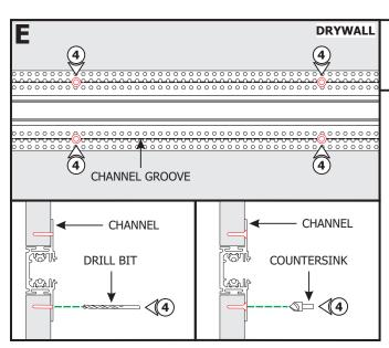
**4:** Place the assembled channel in the drywall cutout. Using the marked joist and mounting strap locations on the drywall, drill and countersink the channel along the groove lines using the provided square drill with countersink bit.
