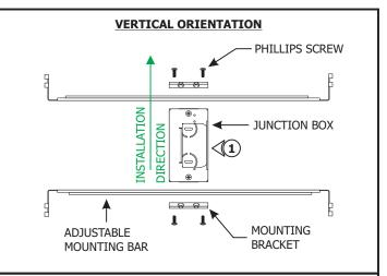
**1:** Mount each adjustable mounting bar to one side of the junction box and secure them with the mounting brackets and Phillips screws provided.
