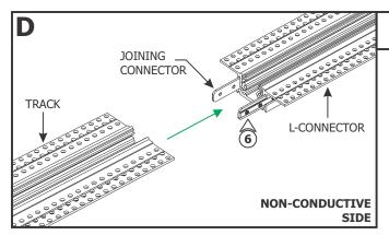
**6:** For the non-conductive side, slide the track over the joining connectors and tighten the remaining set screws.
