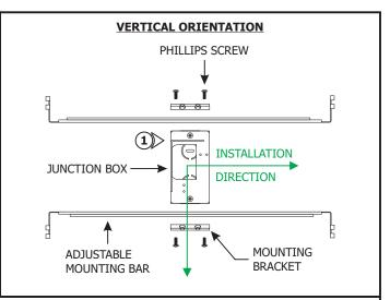
1: Mount each adjustable mounting bar to one side of the junction box and secure them with the mounting brackets and Phillips screws provided.
