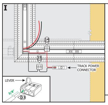
**NOTE:** Follow steps 13 through 19 for connecting the L-Shaped Power Feed as a dual power feed.
