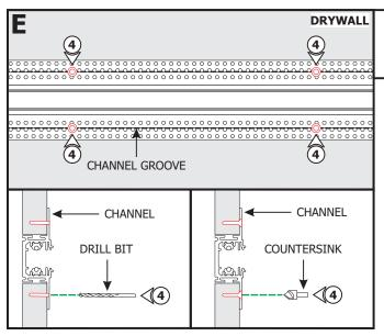
4: Place the assembled channel in the drywall cutout. Using the marked joist and mounting strap locations on the drywall, drill and countersink the channel along the groove lines using the provided square drill with countersink bit.
