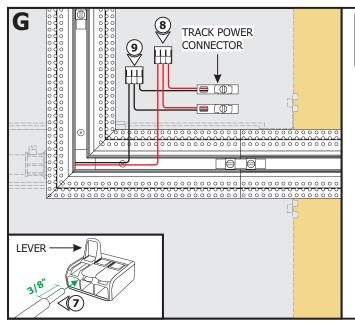
**NOTE:** Follow steps 7 through 12 for connecting the L-Shaped Power Feed a single power feed. Omit steps 13 through 19 on page 4.
