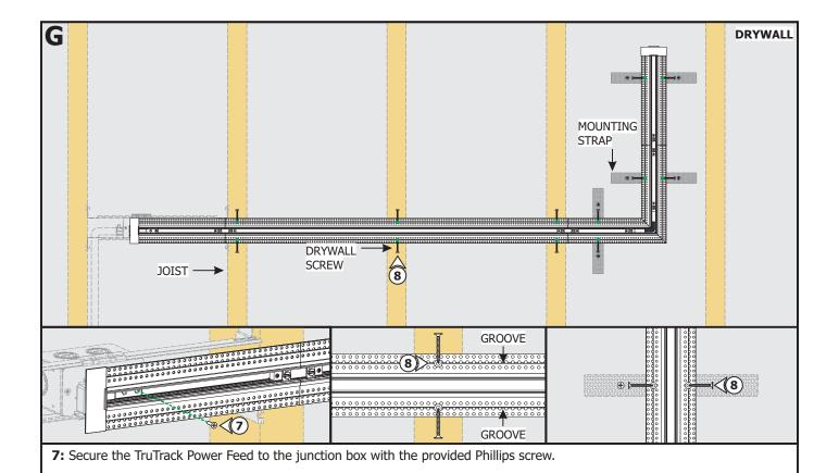
**8:** Properly secure the channel to the marked joists and mounting straps using drywall screws (**DO NOT over tighten**).
