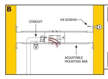
**NOTE:** Adjustable mounting bars mount to studs that are spaced 15" to 24" apart. If the span needs to be shorter than 15", then break the bar arms from dedicated lines.
