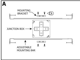
1: Mount each adjustable mounting bar to one side of the junction box and secure them with the mounting brackets and two Phillips screws provided.
