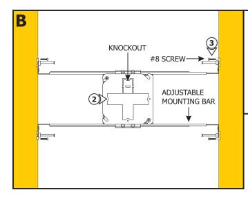
**NOTE:** Adjustable mounting bars mount to studs that are spaced 14.5" to 25" apart.
