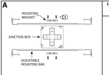
1: Mount each adjustable mounting bar to one side of the junction box and secure them with the mounting brackets and two Phillips screws provided.
