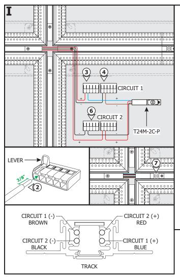
**NOTE:** Depending on the design, discard any unused Power Feed Connectors. Refer to the general wiring diagrams on pages 5 and 6.
