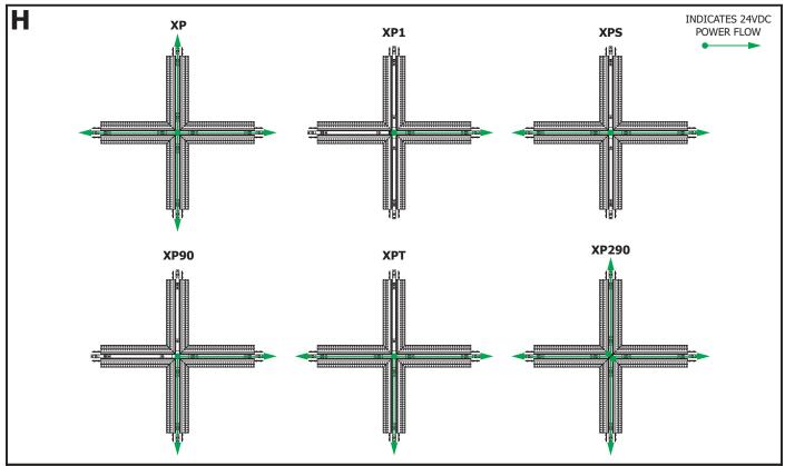
1: The X-Shaped Power Feed joins four sections of track together and conduct power to all channels; all four channels (XP), one channel (XP1), straight through two channels (XPS), two channels in a 90° turn (XP90), three channels in a T-Shape (XPT), and four sections in two 90° turns (XP290).
