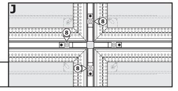
**8:** Depending on the design, repeat steps 2 through 7 to connect the remaining Power Feed Connector to the remaining power supplies.
