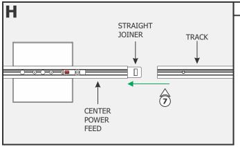
7: Slide the track into the straight joiner.
