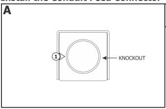
1: Remove the knockout on the back of the Conduit Feed Connector using a flathead screwdriver or other appropriate tool.
