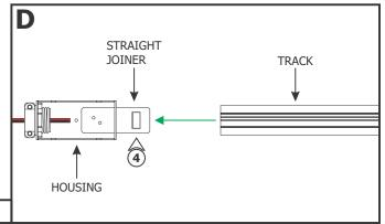
4: Slide the track over the straight joiner on the housing.
