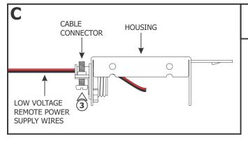
**3:** Install an appropriate 1/2" fitting cable connector to the housing and run low-voltage 24VDC power wires coming from the remote power supply into the housing.
