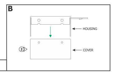
**2:** Remove the cover from the Conduit Feed Connector housing.
