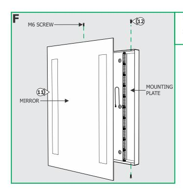
**11:** Carefully place the mirror onto the mounting plate.
