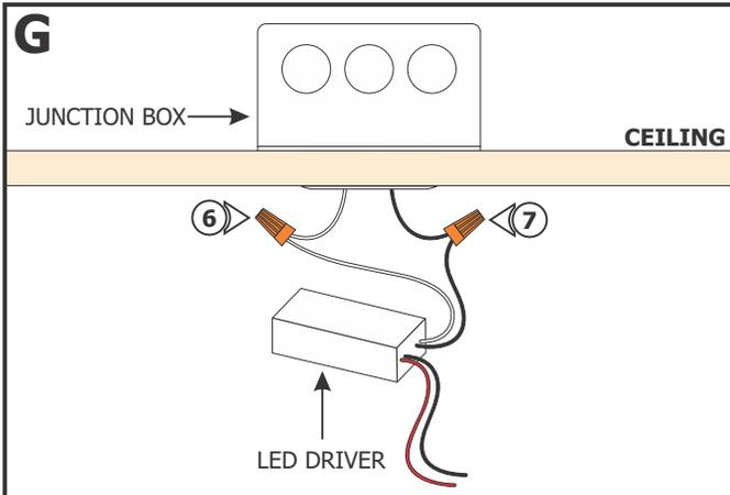
**NOTE:** Steps 6 through 8 are for the 24V power supply included inside the junction box. Omit these steps if using remote power supply.
