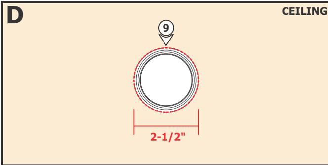
**NOTE:** Vanishing Point Millwork needs to be installed onto a minimum 5/8" to maximum 7/8" thick wood/surface. The cut out slot must be 2-1/2" in diameter.
