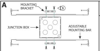
**NOTE:** Adjustable mounting bars mount to studs that are spaced 14.5" to 25" apart.
