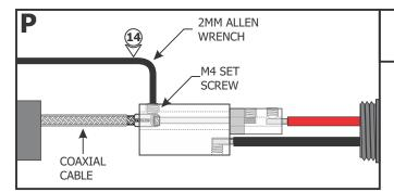
**14:** Use the provided 2mm Allen wrench to securely tighten the M4 set screw until it squeezes the wire ferrule tightly to the coaxial cable.
