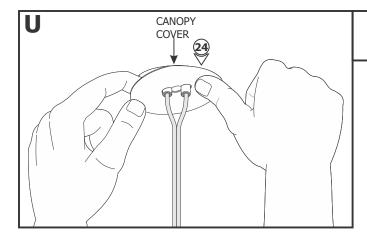
**24:** If necessary, use fingers to push on the perimeter of the canopy cover until it slightly rocks and lift the cover to remove it from the assembly.
