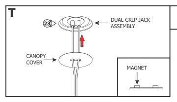
**23:** Place the canopy cover over the Dual Grip Jack assembly. The magnets on the back will keep the canopy cover in place.
