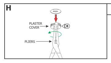
**8:** Use pliers to rotate the plaster cover counter clockwise and remove it. Clean the hole.
