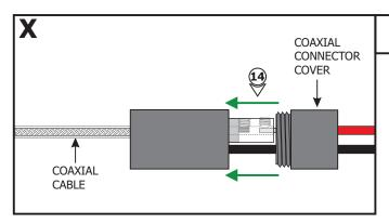
**14:** Replace the coaxial connector cover and tighten into place.
