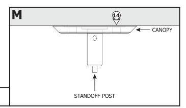
**14:** Place the canopy over the standoff post and magnetically attach the canopy to the washer.
