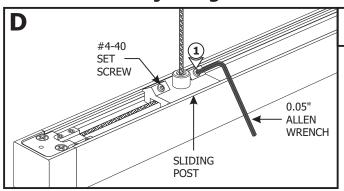
**1:** Loosen (**DO NOT REMOVE**) the two #4-40 set screws on the sliding post with a 0.05" Allen wrench.
