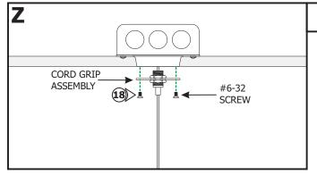
**18:** Mount the cord grip assembly to the 2" plaster ring using two #6-32 screws.
