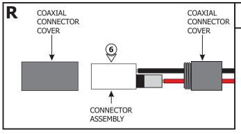
**6:** Unscrew the coaxial connector covers and remove from the connector assembly.
