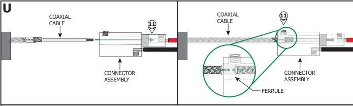
11: Insert the coaxial cable into the coaxial connector until the wires of the center conductor are visible through the M3 set screw hole.
