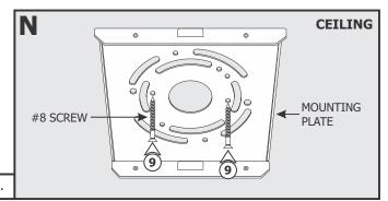
**9:** Secure the mounting plate to the ceiling using the #8 screws.
