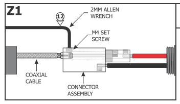
**12:** Use the provided 2mm Allen wrench to securely tighten the M4 set screw until it squeezes the wire ferrule tightly to the coaxial cable.
