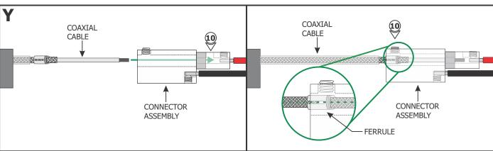
**10:** Insert the coaxial cable into the coaxial connector until the wires of the center conductor are visible through the M3 set screw hole.
