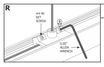
**3:** Place the sliding post back onto the channel and secure it by tightening the two #4-40 set screws with the 0.05" Allen wrench.
