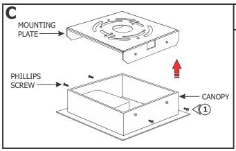
**1:** Remove the four Phillips screws from the canopy to remove the mounting plate.
