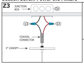
**NOTE:** Omit steps 1 through 4 if using 5" and 6" Surface Mount Canopies. Adjust fixture height by following step 9 on page 8.
