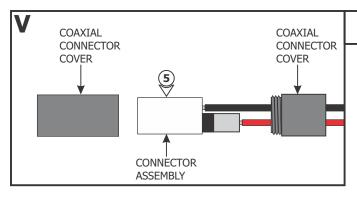
**5:** Unscrew the coaxial connector covers and remove from the connector assembly.
