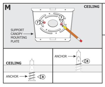
**7:** Mark points through the mounting plate holes onto the ceiling.
