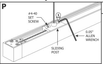
**1:** Loosen (**DO NOT REMOVE**) the two #4-40 set screws on the sliding post with a 0.05" Allen wrench.
