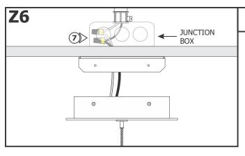
**7:** Place all line voltage wires and wire nut connections inside the junction box.
