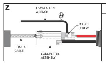
**11:** Use the provided 1.5mm Allen wrench to replace and securely tighten the M3 set screw.
