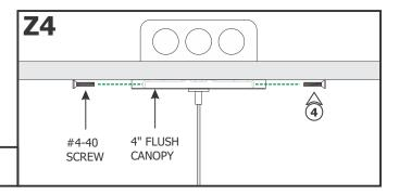
**4:** Align the canopy with the crossbar and secure it with the two #4-40 screws using a 1/16" Allen wrench.
