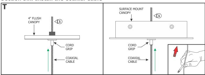
**NOTE:** If cable is curled or kinked, straighten by holding between the shaft of a screwdriver and thumb and pulling the cable through (see inset).
