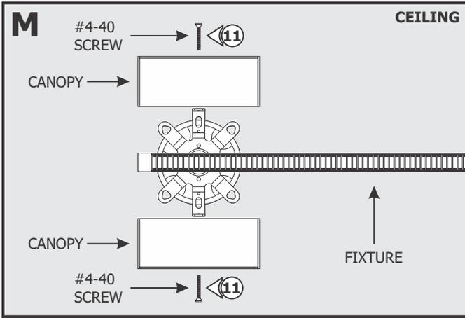
**11:** For 4" Square Canopy installations, place each canopy piece against the fixture and align the canopy holes with the crossbar holes. Secure the canopy pieces in place with the two #4-40 screws and 1/16" Allen wrench provided.
