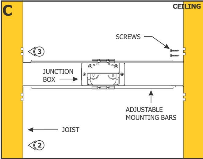
**NOTE:** The adjustable mounting bars mount to studs/joists that are spaced 14.5"-25" apart.
