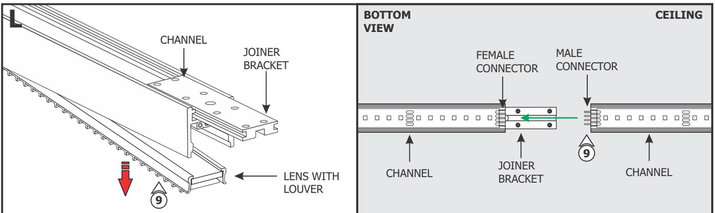
**NOTE:** Omit steps 9 and 10 if the channel is made out of a single piece (120" or less).
