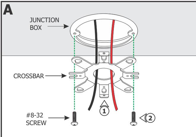
**NOTE:** Remote power supply must be installed within 40ft of junction box. Ensure remote power supply wires are present in the junction box. Refer to instructions provided with the power supply.
