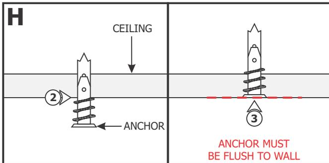
**NOTE:** Steps 2 and 3 are for drywall mounting. Omit these steps if mounting the clips to a wood surface directly.
