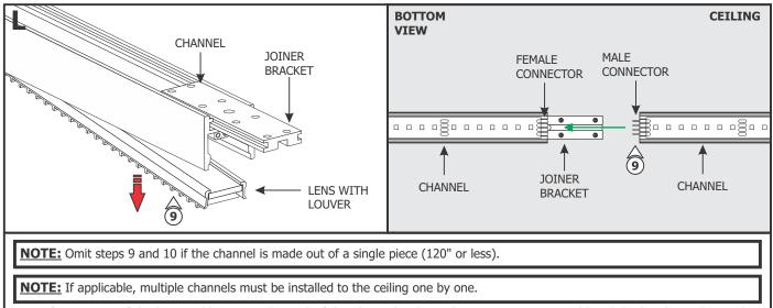
**9:** Lift a section of the lens and louver at the end of the channels where the connectors are visible. Slide the channel over the joiner bracket making sure that the male & female connectors mate properly. Push the lens and louver back into the channel.
